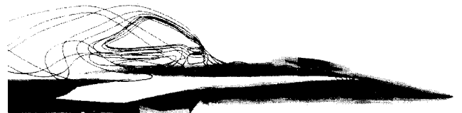
Fig. 12 Wing/fuselage predicted LEX vortex; M_\infty = 0.243 , \alpha = 30.3 deg, Re_c = 10.0 \times 10^6 .
